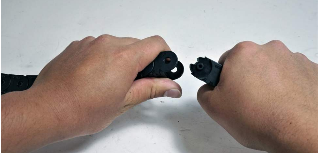
Use both hands to twist and disconnect the drag chain links.
