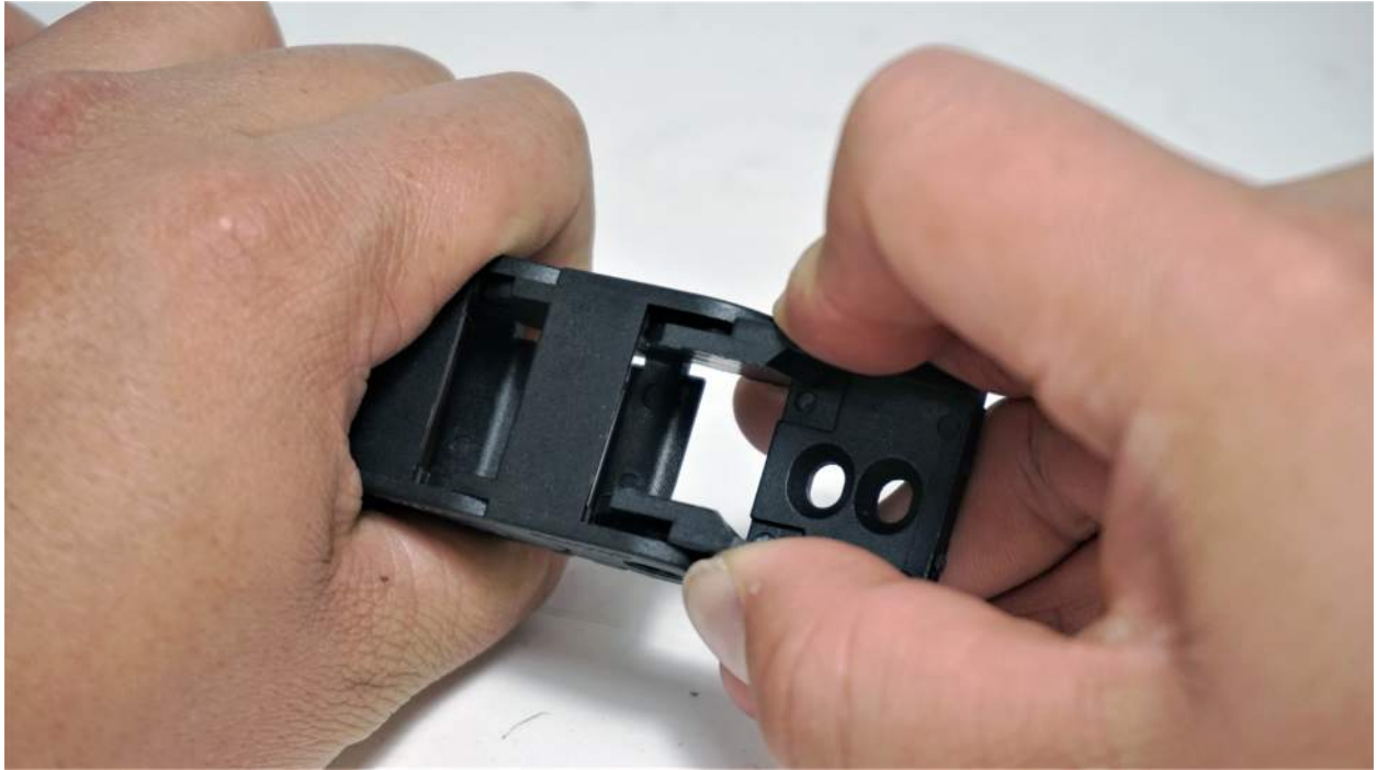
For the pin-type end link, squeeze the two sides of the link together, then twist and pull to disconnect
