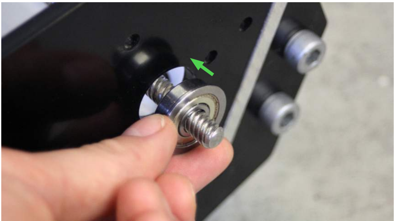
Push the coupler all the way into the bearing, and retighten screw
