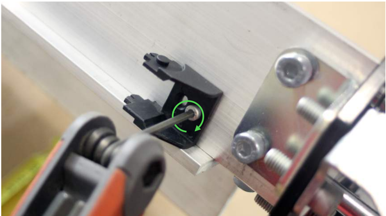
Use an M4 nylock nut on the other side of the aluminum angle if needed
