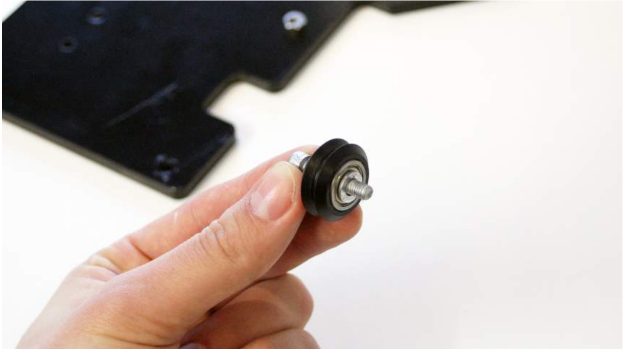
V-wheel sets with a washer to keep the v-wheel spaced from the gantry plate
