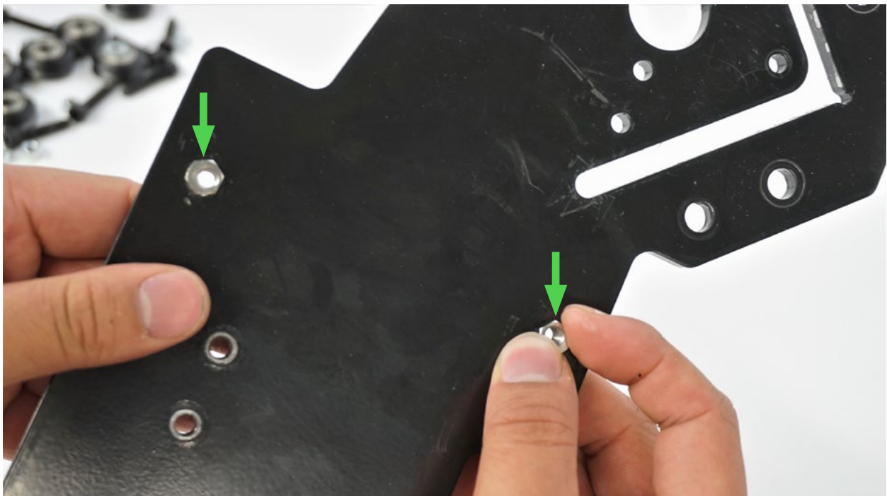
Install the eccentric nuts into the top two holes.
