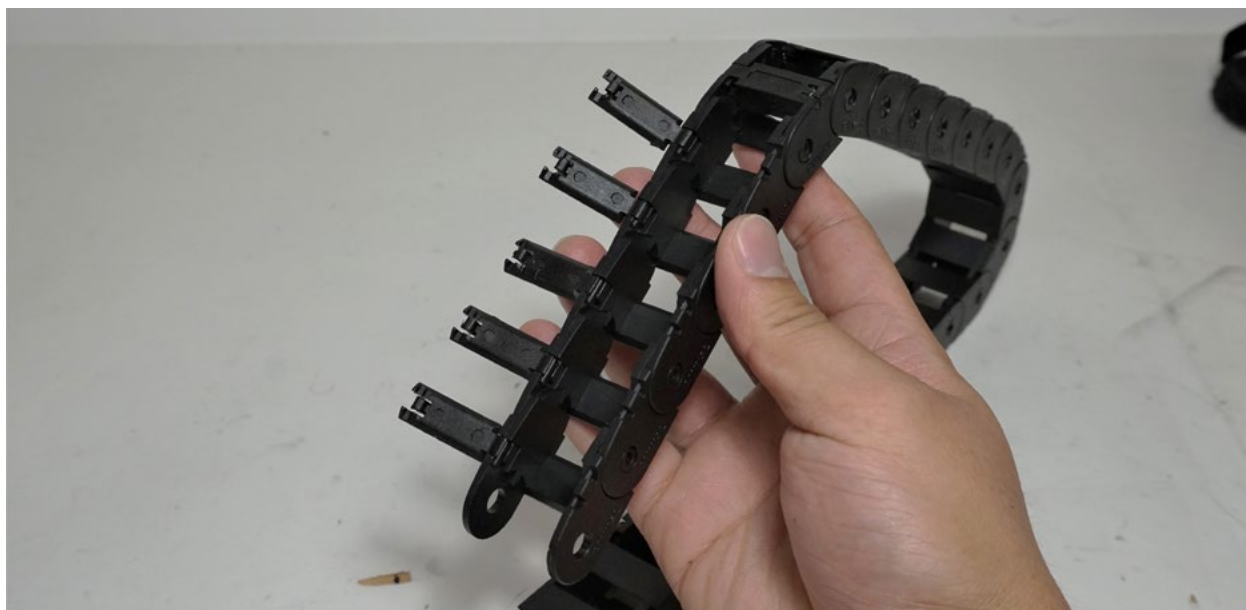
Unclip the tabs on the drag chain
