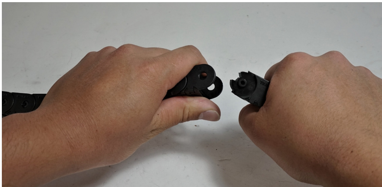
Use both hands to twist and disconnect the drag chain links.
