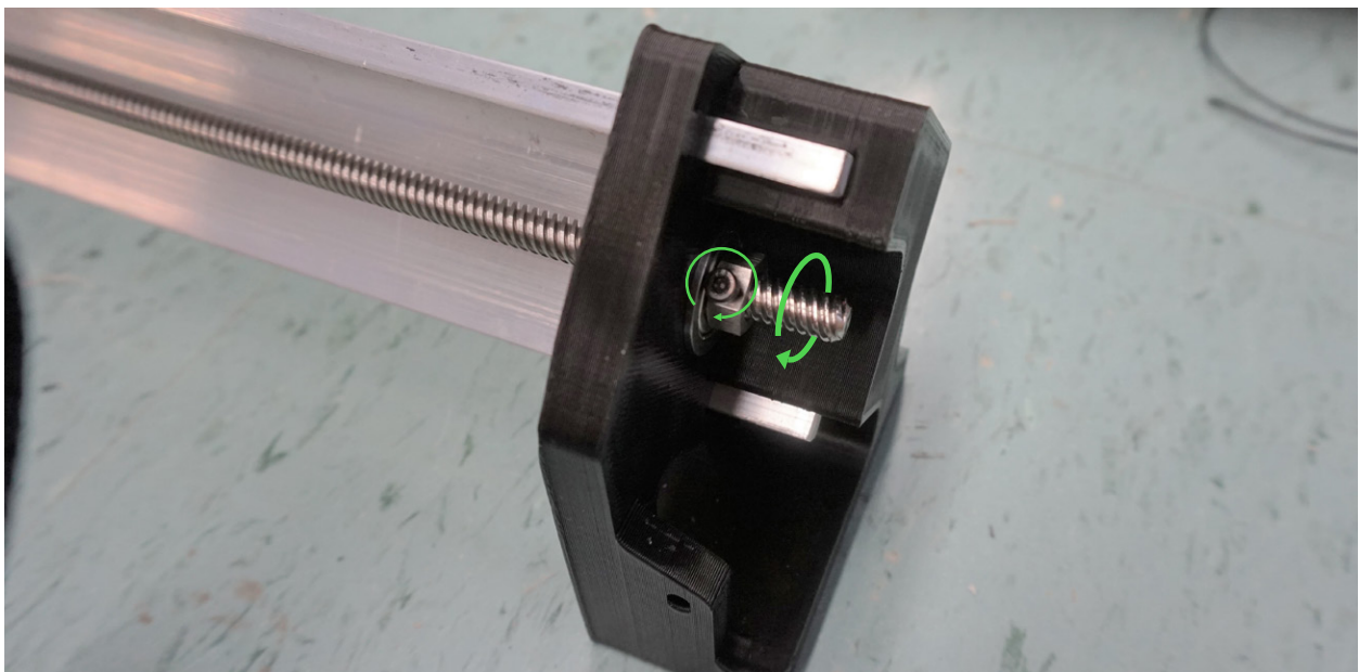
Thread on the ACME lock nut, making sure it's tight against the bearing before tightening the screw to secure
