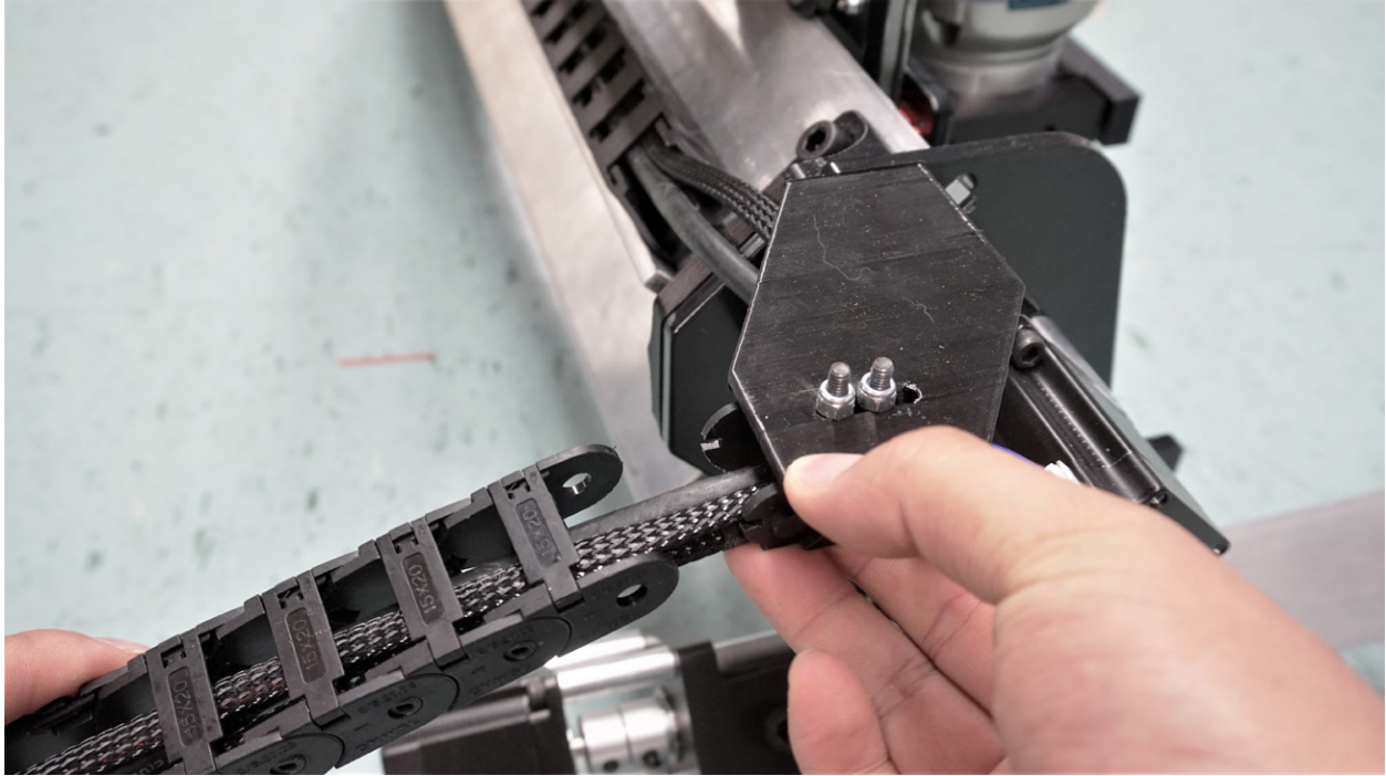
Grab the Y-axis drag chain and insert the X and Z-axis motor cables and router cable
