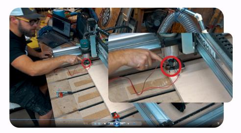
We're using Sienci's Autozero Touch Plate to find 0 for our project. We've got the bit centered over the touch plate inside the square target zone. We've also hooked up the magnet to the collet nut for conductivity in the next steps.
