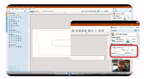
Within this menu, you're able to select what type and size of the bit is being used. We've selected a 1/8" down cut endmill. You can adjust the depth of cut, and if you select "edit" it will open up speed and feed settings for the chosen bit.
