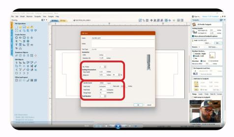
Within this menu, you'll find all the settings you need to adjust the feeds and speeds for the selected bit. We've chosen a .25" pass depth, 100 ipm feed and 75 ipm plunge rate.
