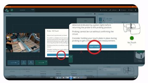
Once your desired axis' and bit type are selected, we hit "probe." gSender will wait for us to touch the autozero touch plate to the bit in the router to ensure conductivity. Once it has detected the touch, we can click on "Start Probing." It will cycle through the selected axis, and once complete move to 0.
