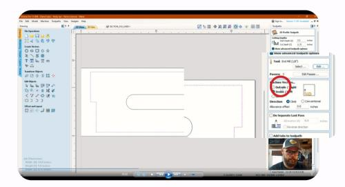
Selecting "outside" for the machine vector will ensure the bit follows the outside of the path selected. This is what we need for this part of the step stool.
