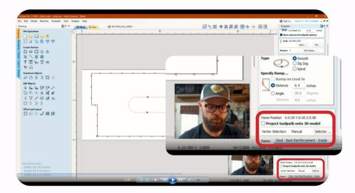
We'll rename the toolpath to include "inside" so we can tell them apart. We'll also drag the inside to the top of the toolpath list so it is cut out first, and then the outside toolpath second.
