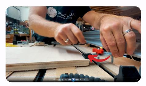
Make sure your workpiece is square to the machine (assuming it needs to be) and clamp your piece down with the appropriate work-holding method. We've chosen Sienci's metal clamps as we have lots of space around the workpieces to secure them without interfering.
