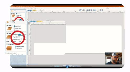
We used Vcarve to create this project. Create a new file, the dimensions can be changed at any point so it's not super important that the size is correct right now.
