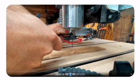
If you haven't already done so, secure the chosen bit in the router. We've chosen a 1/8" down-cut end mill (we later changed to a 1/8" compression bit as they do a solid job of cutting all the way through most materials). be sure to tighten the collet with the proper 2 wrench method.
