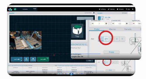
We've selected "XYZ" from the Probe menu because we need to find all 3 axis' 0 locations. We chose "tip" from the drop-down menu because we're using Vbits. For end mill bits, "auto" can be selected.
