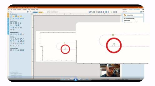
Again you can decide to add tabs automatically or manually. We chose manual and dropped in 4 tabs to hold the centre piece in place.
