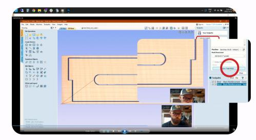
Make sure the toolpaths you want to be saved have a check beside them. We've selected "all visible toolpaths to one file" so the inside and outside toolpaths will be saved to a single file. Once loaded, they will run one after the other to complete the cut. Repeat all steps for each of the other pieces for the step stool.
