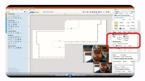
Adding ramping will ensure our bits aren't subject to unnecessary wear, so we'll check that on.
