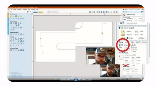
By ramping out toolpaths it will save unnecessary wear and tear on the bit, so we'll check that on and set to .5 in.
