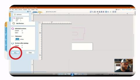
A menu will come up displaying stats for closed and open vectors within the sheet. Once you click on "join" any open vectors will now be closed. This means all segments will be joined instead of individual segments as they were.
