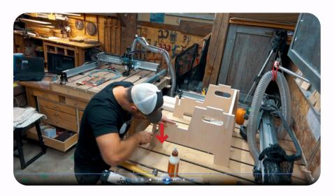
Some of the slotted parts may be a little wee bit tight when assembling. That's where files, sandpaper, and a rubber mallet come to the rescue. I dry fit everything before gluing all the pieces together.
