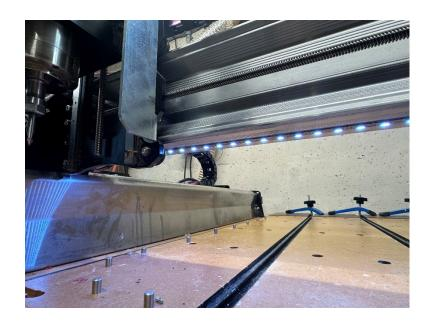
14. Power strip attached to bottom of X gantry. Strip had self-adhesive strip but I added hot glue in spots
