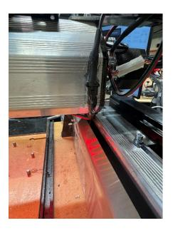
12. Secure cable to the back of the X gantry (Ugly hot glue job)
