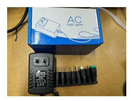
The power adapter includes multiple tips. We are using the DC jack (green) on the right
