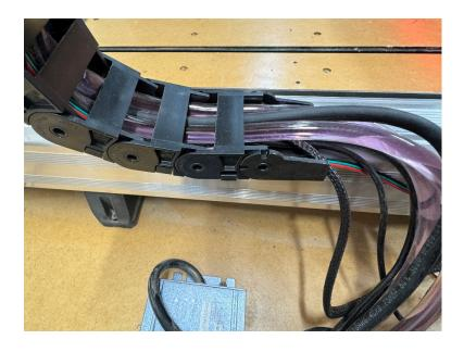
10. Run the LED extension cable into the drag chain
