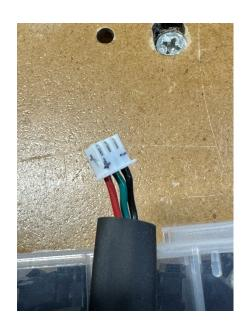
5. Install JST-XH 2.5 3 terminal male connector to LED extension cable. Note wire configuration on board.
