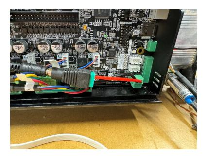
4. Connecting the LED PWR to the power supply
